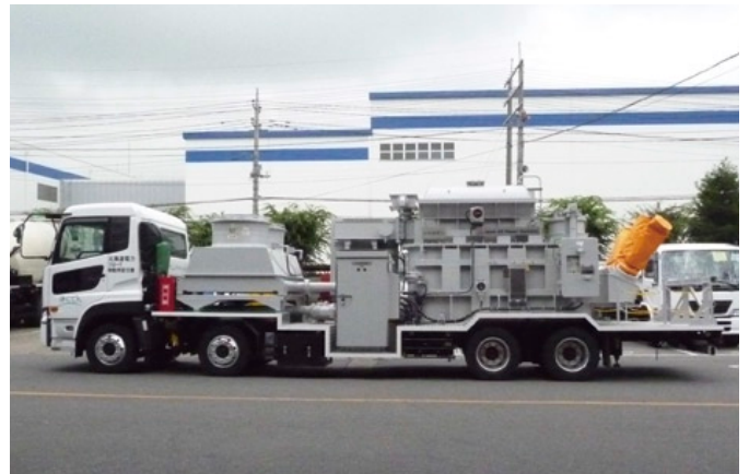
64.5kV 17MVA Transformer for Mobile Substation
